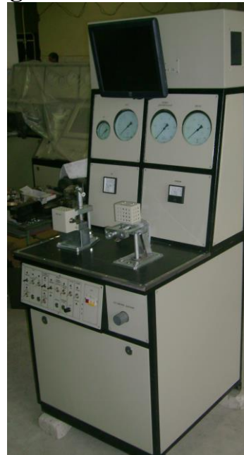
IS-210.760/A (parking brake control unit (BUST))
