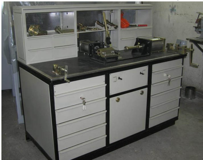
WB-018 (pneumatic actuator for electric-box coupler subway car, connection hose P32, P34, P21, P23: assembly/disassembly)
