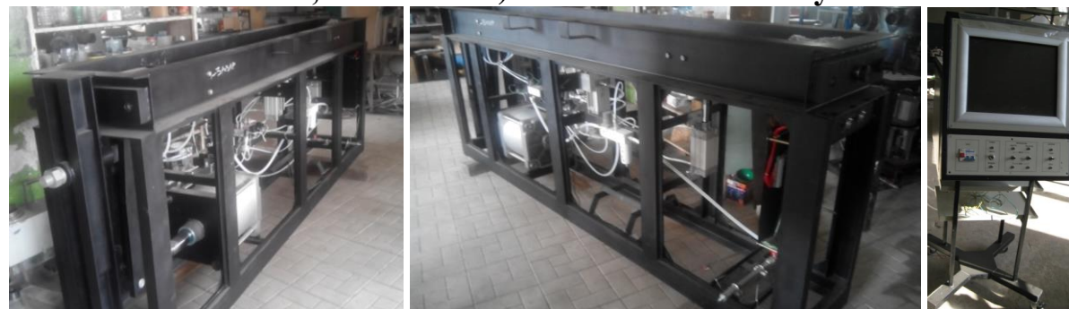
IS-177/A (brake linkage regulator (Slack adjuster) types PTPИI-675, PTPИI-675M, PTPИI 574Б). Under tests currently!
