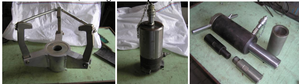
SDT-725 (clutch generator puller). Under tests currently!
