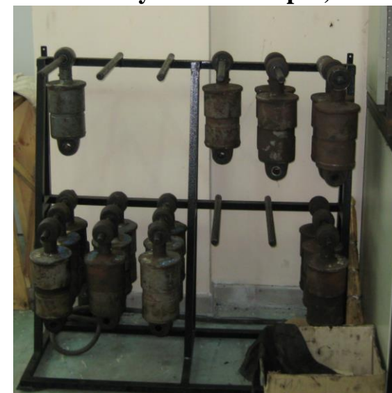
CH-403 (special stillage store for hydraulic damper)
